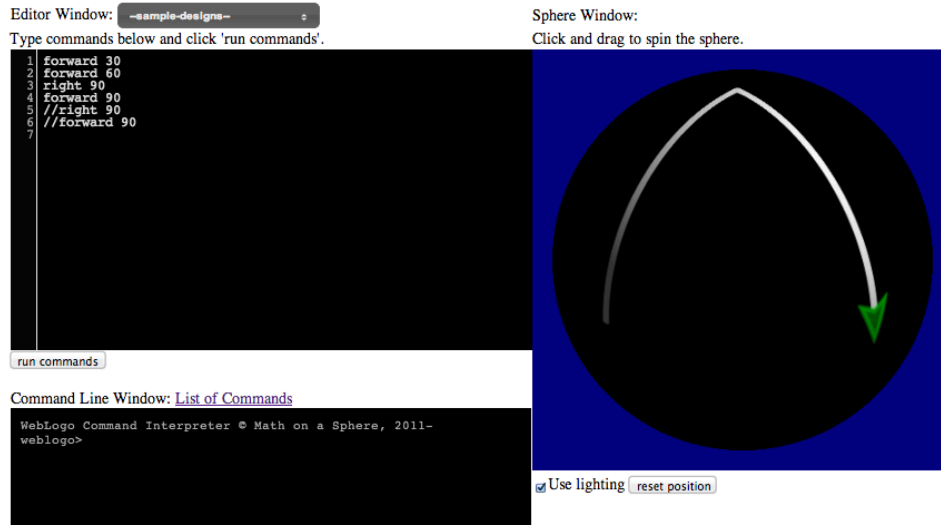
Figure 4. You can use // to comment out lines of code. Instructions that follow // are ignored by the turtle.
